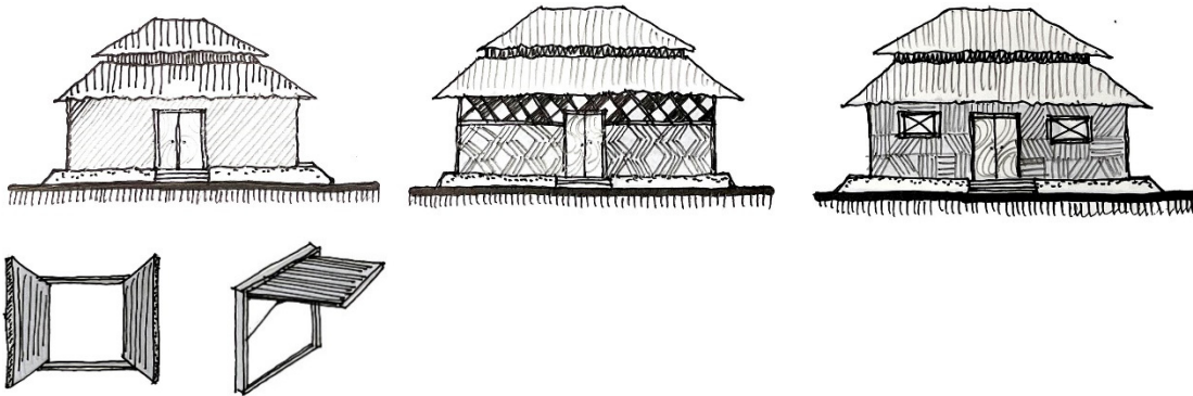
Figure 11: Limited and symmetrical opening on the external facades
