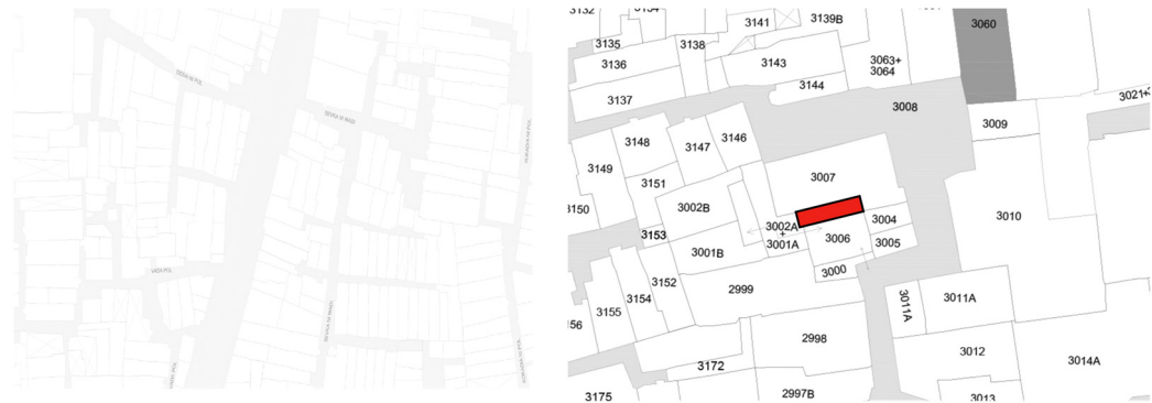
Figure 1 (a): Typical layout of Pols spread across the main road in old city of Ahmedabad, Gujarat showing dense urban fabric of community housing. (b): Pol houses layout seen in Fad Pol in house 3003 is marked in red which is documented under measured drawing activity for study purpose.
